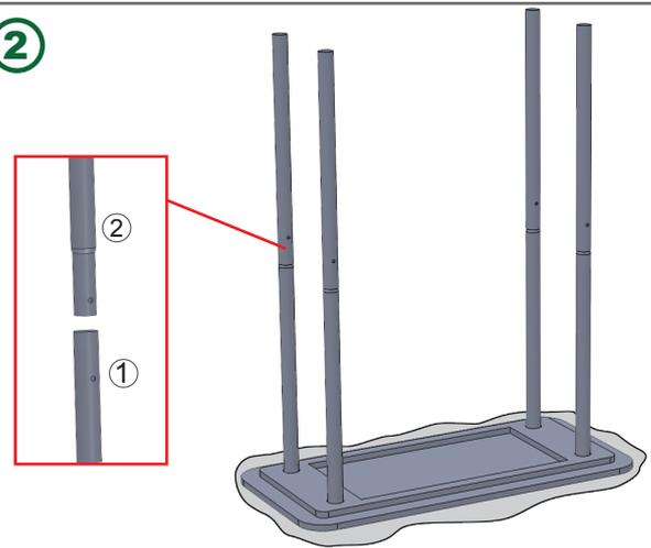
Connect the Pipe #1 and #2, inserting them into the slots in base
